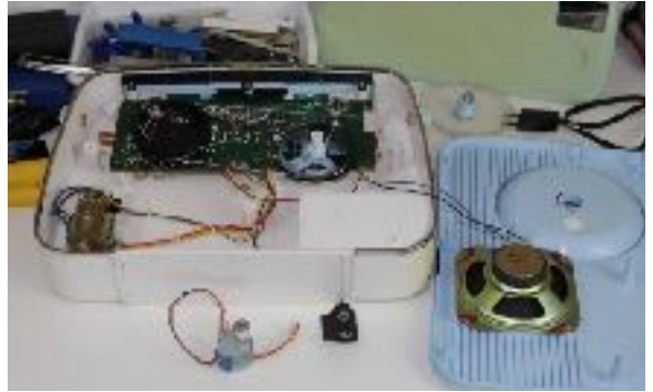
The large speaker on the case top cover has been removed to make space for the stepper motor.
