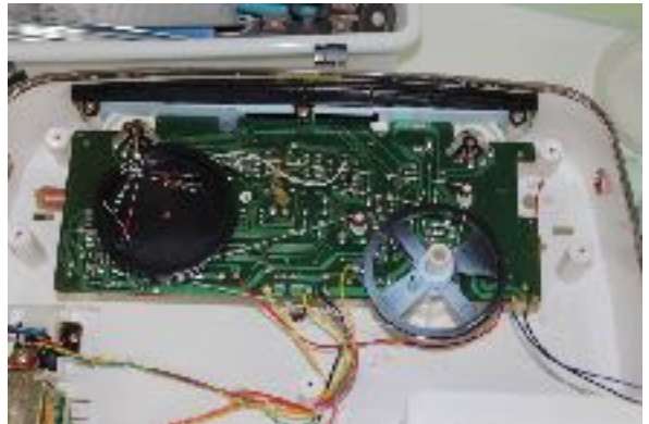
The tuner mechanism: the variable capacitor to the left and the tuner knob to the right.
